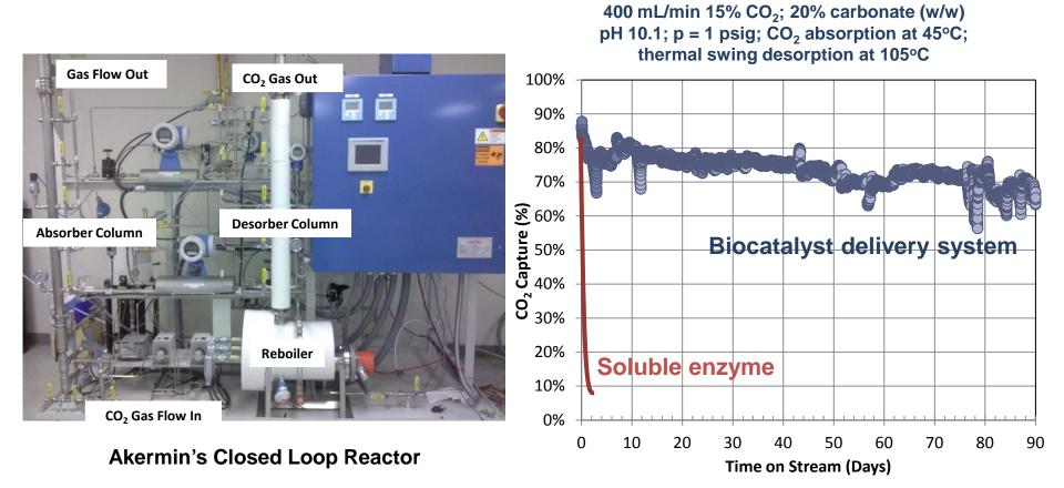
>20 million CO<sub>2</sub> molecules hydrated by one CA molecule over 75 days Initial performance >400 kg CO<sub>2</sub> captured per day per kg of CA
