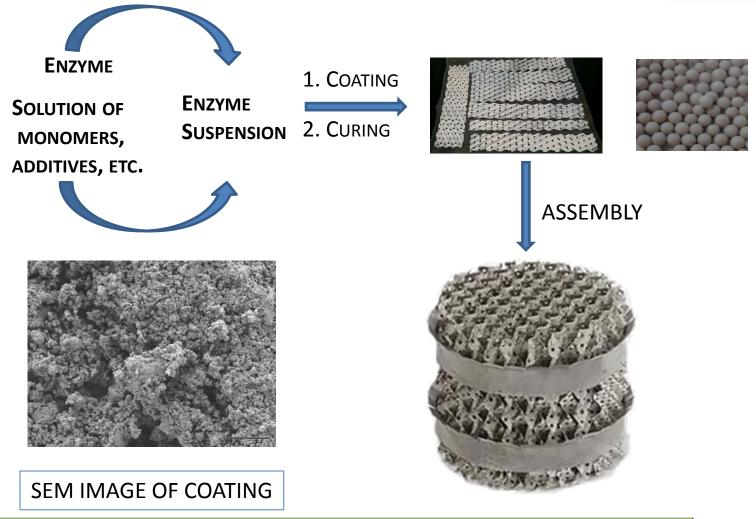
Akermin developed several proprietary approaches to exhibit CA at gas/liquid interface of absorber column
