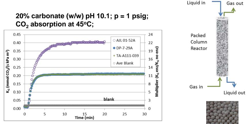
$K_{G}$  per packing area, lab-scale test reactor interfacial area ~ 30%
